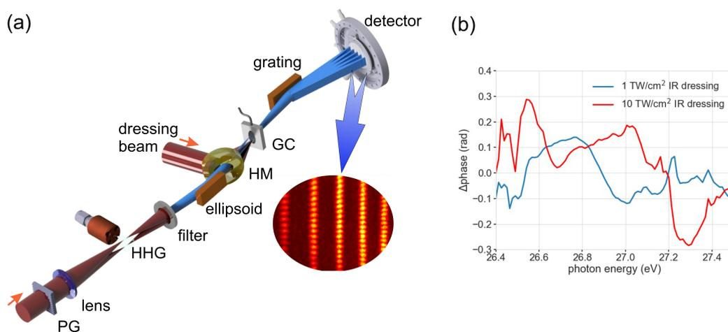
Figure 1: **a.** Scheme of the experimental setup. PG: phase grating; HM: holey mirror; GC: gas cell; HHG: high harmonic generation. **b.** Dependence of the phase response measured in Ar around the 4p Fano resonance on the dressing intensity at the temporal overlap between the pulses.
