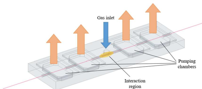
**Figure 1:** Multichamber chip design. The central gas-laser interaction region is supplied with gas from the top. The four chambers on both sides are connected to vacuum pumps.
