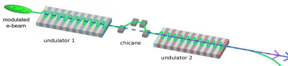
**Fig. 1: Schematic representation of the two-pulse technique.** The split undulator technique creates pairs of attosecond pulses from a single ESASE current spike.
